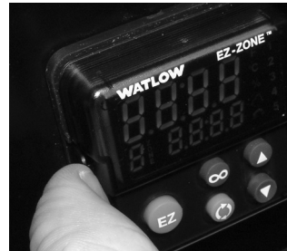
Pull out the tab on each side until you hear it click.
